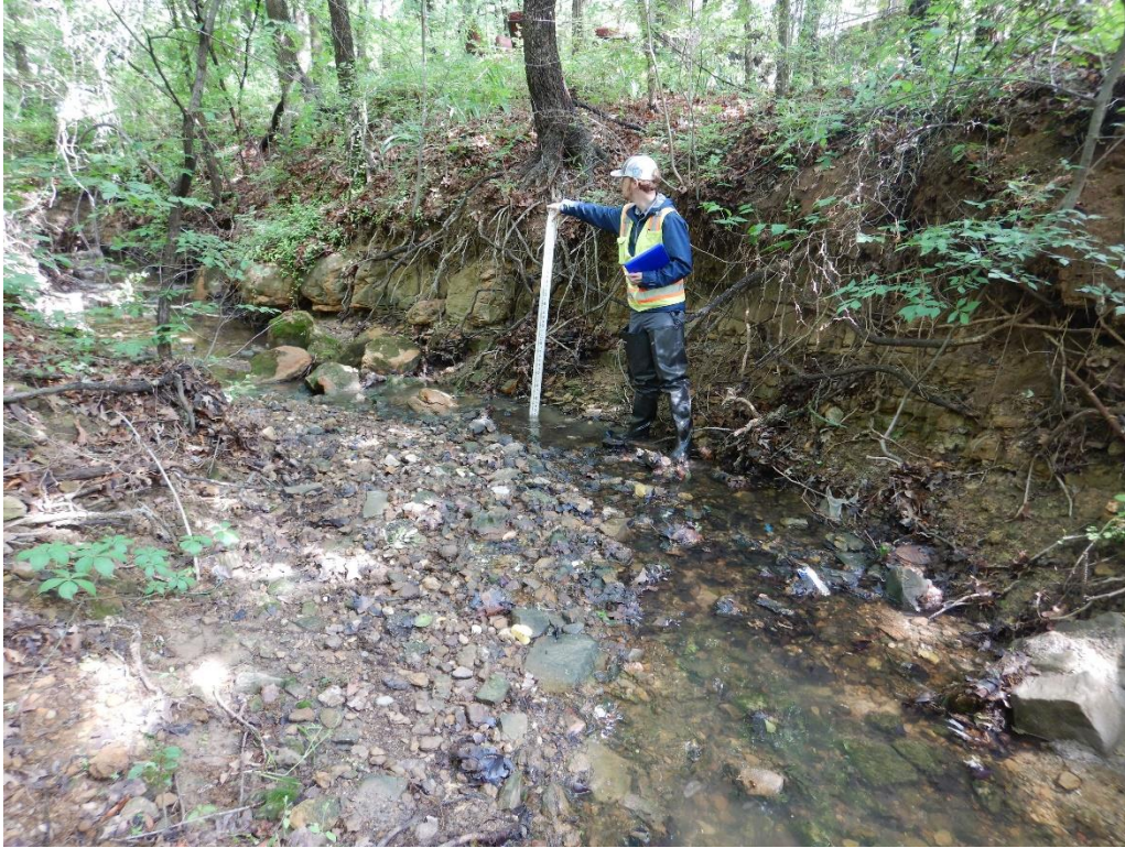
Station 16+25 - Looking downstream, this photo shows representative conditions of the channel in this area. Bank erosion may impact the backyards of homes ( Area of Concern #11 ).
